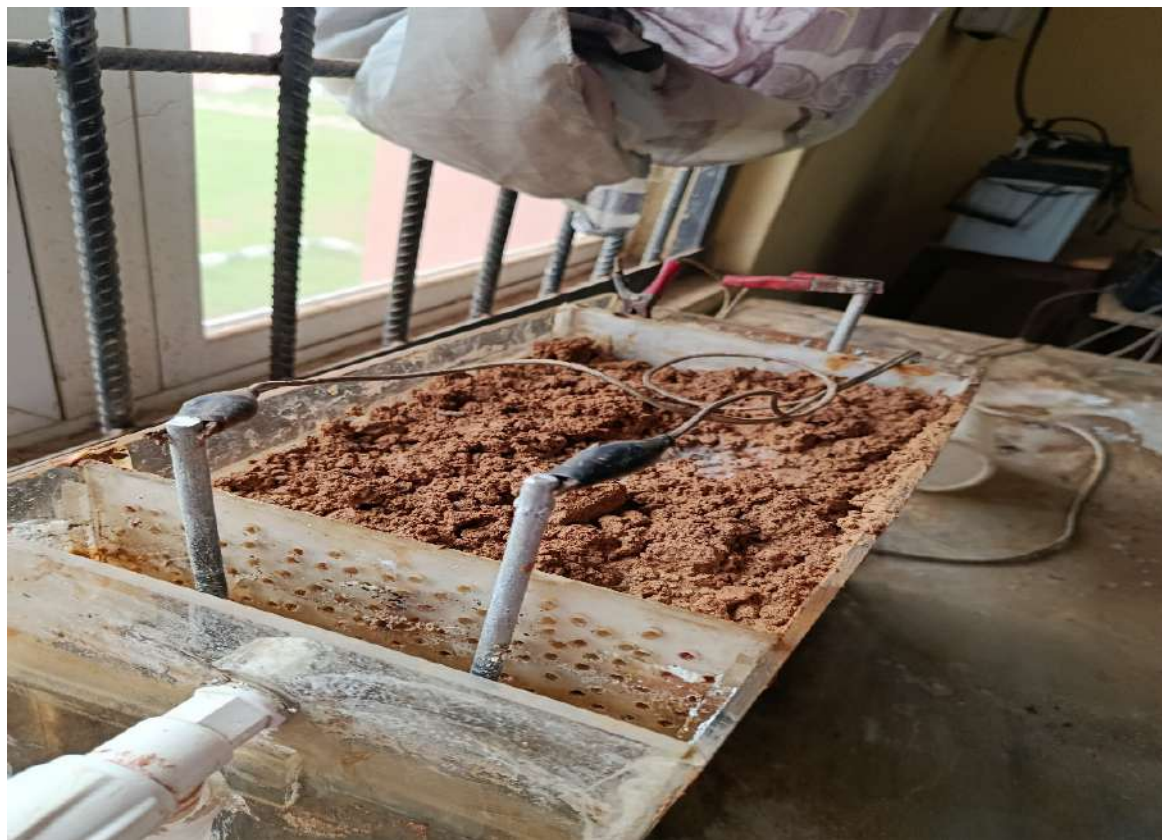
Plate 1: EKR setup for Aluminium electrode
