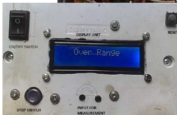
Figures 4a and 4b: The designed and Constructed LC Meter Assembled in Casing
